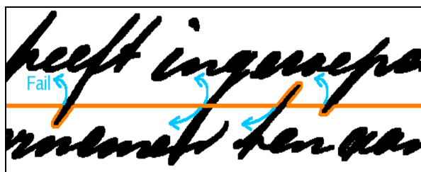
Figure 3: The “droplet” technique generates curvilinear line separators that preserve the ascenders and descenders. Occasionally, when both search directions fail, ink cuts are applied.
